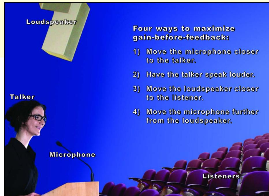
Figure 4 Maximum Gain-Before-Feedback
