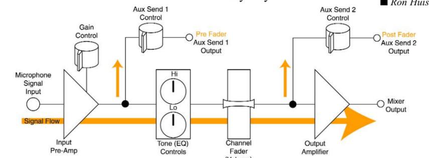
Figure 5 The path of a signal through a mixer.
