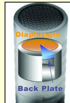
Figure 2 Electret Microphone
